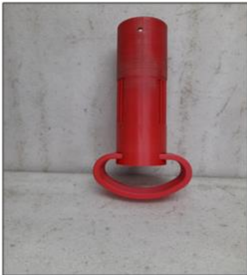
Fig.8: Pylon and shock absorber 3D printed
