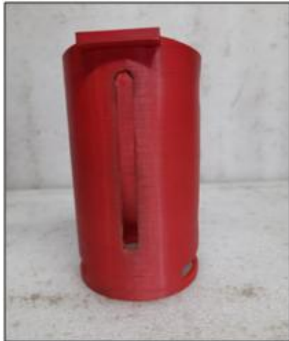
Fig.7: 3D printed shank part
