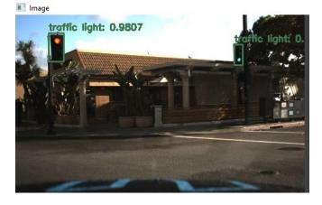
Traffic light recognition was accomplished in the self-driving automobile employing object detection, allowing for accurate analysis and reaction.
