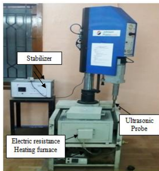
Fig. 1 – Experimental setup for fabricating Al– Al_2O_3/B_4C nano composites.
