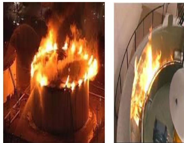
Figure: RIM SEAL FIRE
