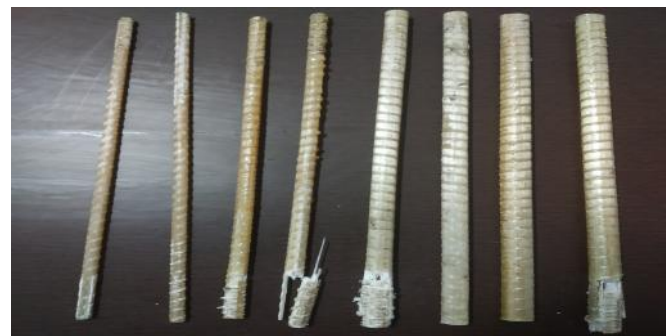
Fig. GFRP after testing on UTM machine
