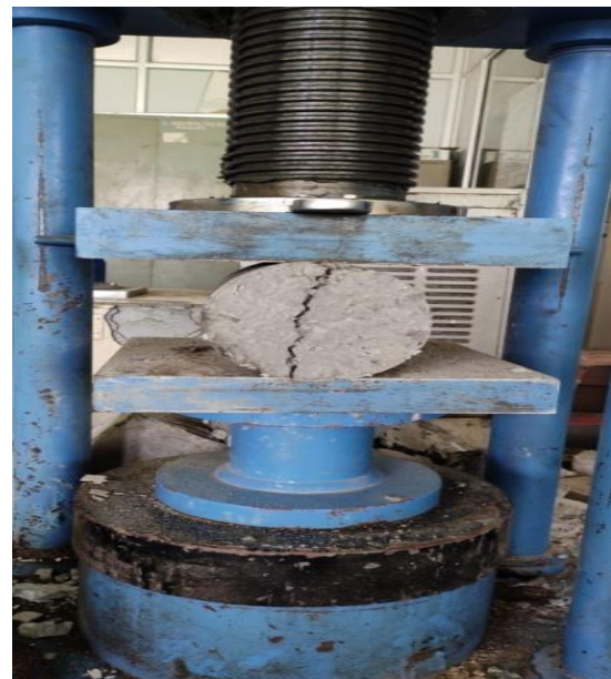
Fig.-2 Splitting tensile strength setup
