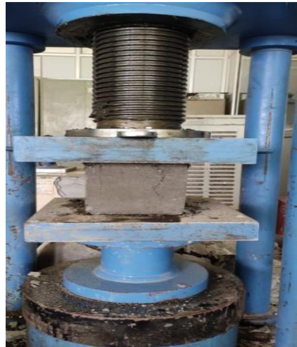
Fig.-1 Compressive Strength setup
