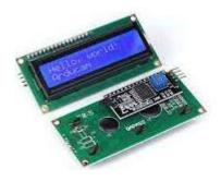
The LCD display with I2C interface is a popular output device that uses the I2C protocol for easy integration with microcontrollers. It features a high contrast ratio, adjustable brightness, and a programmable character generator for custom characters and symbols. The display typically
