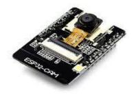
The ESP32-CAM is a low-cost development board that combines an ESP32-S module, camera module, and microSD card slot. It features a powerful dual-core 32-bit processor that can run up to 240 MHz and built-in Wi-Fi and Bluetooth connectivity. The board includes a variety of peripheral interfaces, such as SPI, I2C, UART, and PWM, making it easy to connect to external devices. The camera module included on the ESP32-CAM is a OV2640 camera
