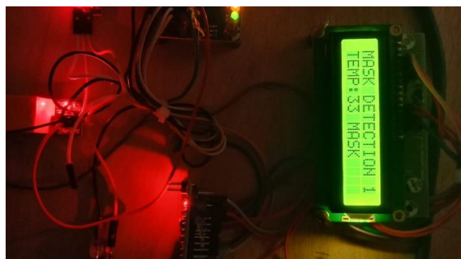
Fig.11 LCD Display Output for Mask Detection
