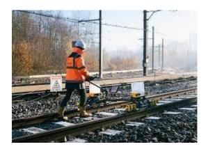
In ultrasonic testing, faults are found using ultrasonic waves, which are sound waves with a frequency between 2-4 MHz. A tiny piece of piezoelectric crystal is mounted in the probe, which is moved over the rail or weld, and it generates, transmits, and receives the waves from the rail or weld.
