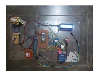
The IOT assembly consists of transformer, resistor, capacitor, Radio Frequency Identification (RFID), Wi-Fi module ESP 8266, GPS module, GSM module, Micro controller, Accelerometer, MQ3 sensor, LCD display.
