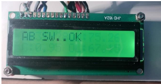
Figure 4.No fault in AB Switch
