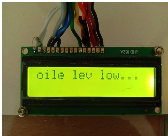
Figure6.Reduction of oil level indicator
