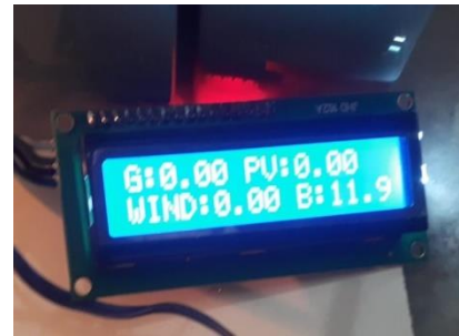
Figure 6.1 : Status of power sources
