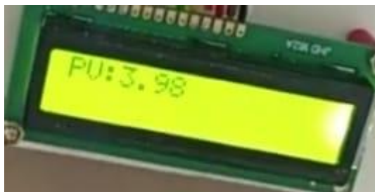
Figure 3.Measured Voltage Level Of The PV panel
