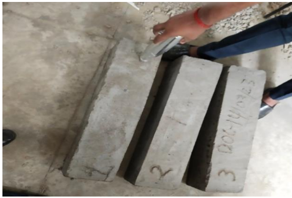
Fig. 8 Rebound hammer test
