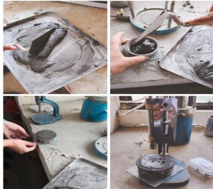
Fig.2 Standard Consistency & Setting time
