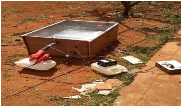
Figure.1.6 Solar Air Heater
