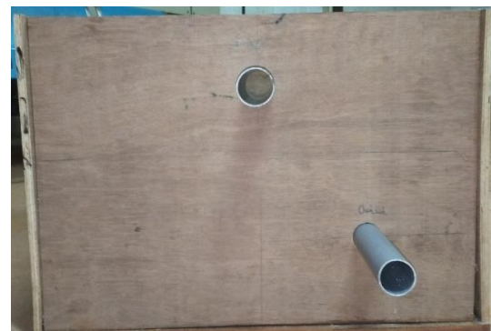
Figure.1.2 Inlet And Out Let Pipe
