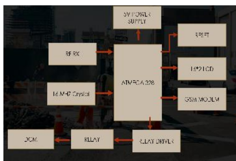
Fig -5 Block Diagram of Implementation of Smart Helmet
