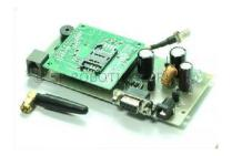
It can be used to send and receive SMS or make/receive voice calls. It can also be used in GPRS mode to connect to internet and do many applications for data logging and control. In GPRS mode you can also connect to anyremote FTP server and upload files for data logic. This GSM modem is a highly flexible plug and play quad band GSM modem for direct and easy integration to RS232 applications. Supports features like Voice, SMS, Data/Fax, GPRS and integrated TCP/IP stack.
