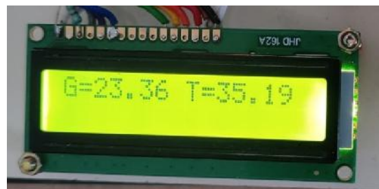
Figure 7. (G-Gas, T-Temperature) After attaining these values the fan & water pump will be turned ON.
