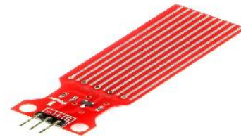
Figure.1.8 Water Level Sensor
