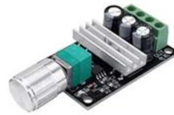
Fig 4.4 DC Motor Speed Controller
