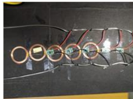
FIG 18 Placement of the coils on the road to transmit power
