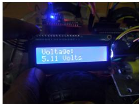
FIG 23 LCD Screen displaying received voltage value
