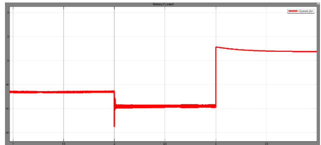
Figure 14: Current waveform for EV Battery
