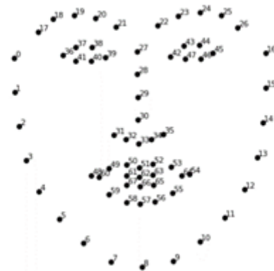
Fig.3: Facial Landmark Detection
