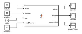
By implementing these calculations, we can precisely determine the sun's position at regular time intervals throughout the simulation. This information serves as the basis for evaluating how solar panels should be oriented to capture the maximum sunlight.
