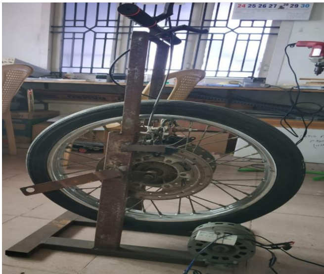
Fig 2. Fabricated model of Frictionless Braking System
