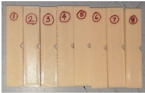
Fig. 6: Impact Test on Specimen
