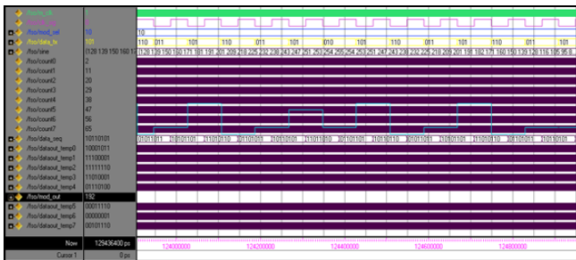
Fig:6 Simulation result of BPSK Modulation
