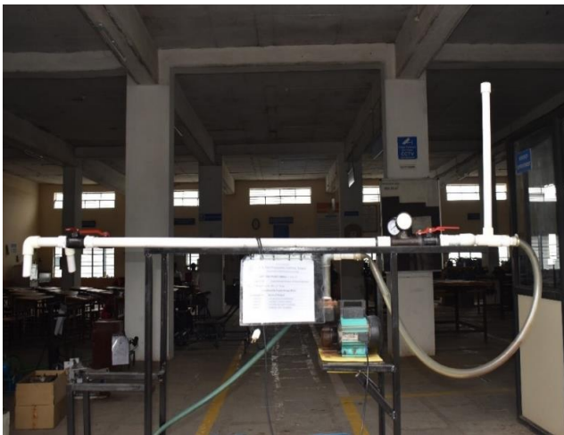
Fig. 2 Experimental Set up of Water Hammer Test Rig
