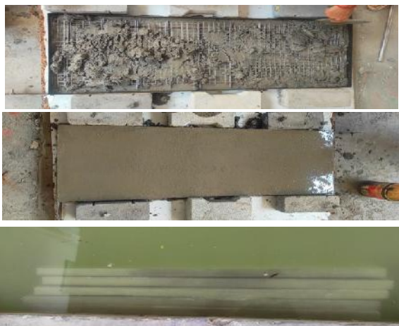
Preparation of Mould and Casting of Slab as Shown in fig
