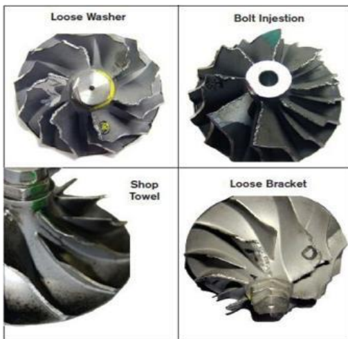
Bad condition of Turbocharger component
