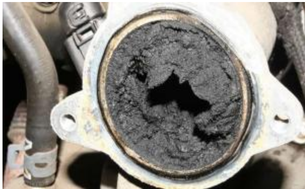
Bad condition of EGR
