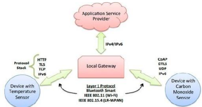
Figure 1.3 Devices to the gateway communication model
