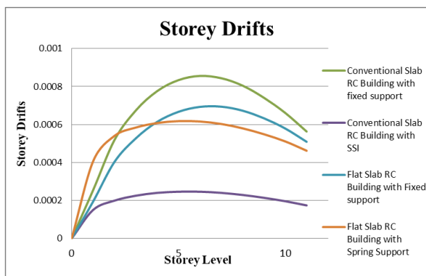
Figshows the Storey Drifts in X-direction for Conventional & Flat Slab building with fixed and spring support
