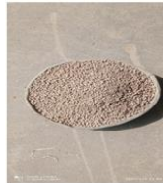
Fig 3.2 Sintered flyash aggregate (4-8mm)
