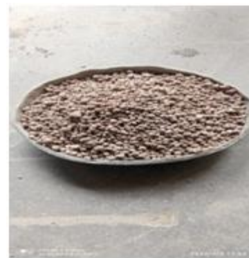
Fig 3.3. Sintered flyash aggregate (8-16mm)
