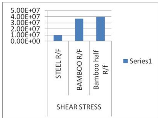
Fig.2.2 comparative shear stresses of steel with Bamboo reinforced concrete
