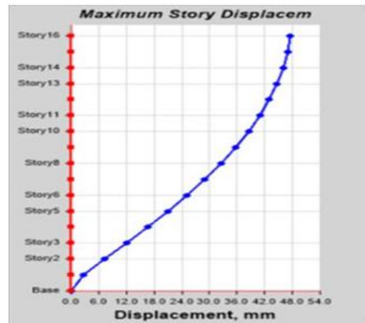
Fig6 Moment Resisting Frame with Steel X Bracing System (Model2)
