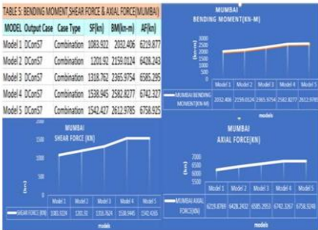
Fig 20 Graphical Representation of Mumbai Models for Drift Table 8 Bending Moment shear Force and Axial Force Comparison
