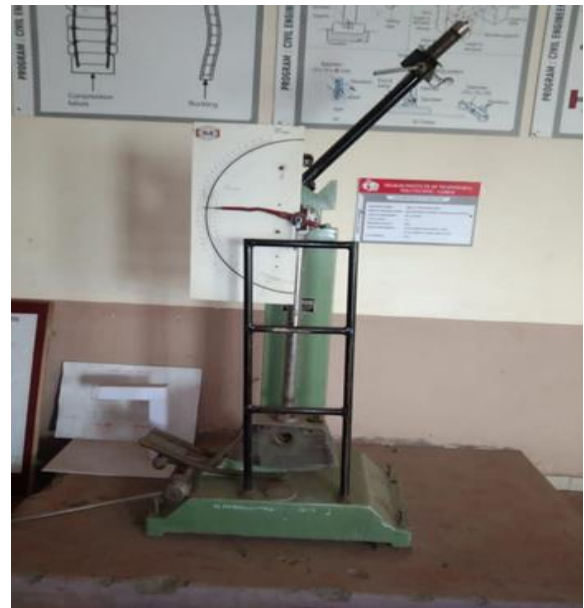
Fig. 6 Charpy impact testing machine
