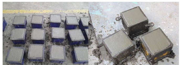
Concrete cubes to be casted in the mold
