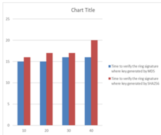
Figure: Graphical representation of the time required for the service provider to verify the ring signature where key generated by MD5 and SHA256
