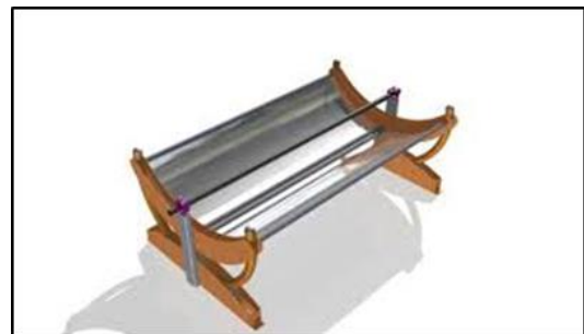
Figure The constructed Trough Collector
