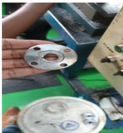
LOCKING PLATE AFTER DRILL
