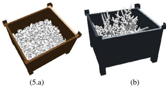
Figure 3: Virtually filled bins with different automotive parts using physics simulation.
