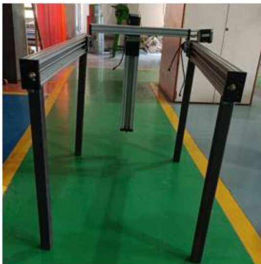
Fig 2.10: Completed Z-axis attachment
