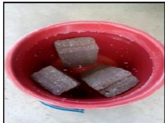
BRICKS WERE IMMERSE IN TO WATER
