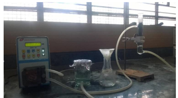
Fig 5.2 continuous operation using peristaltic pump
