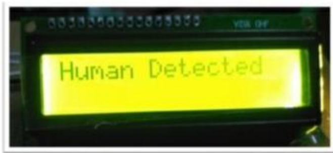
Fig :- Human detected by PIR Sensor
