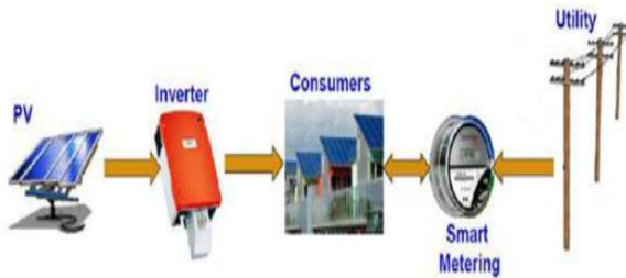
Fig-2: Grid tie solar system
