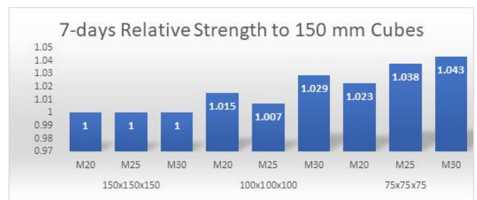
Fig.5: Effect of specimen size on Relative 7-days compressive strength of concrete
