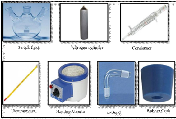
Pic.2: Components used for Fuel Extraction Process
