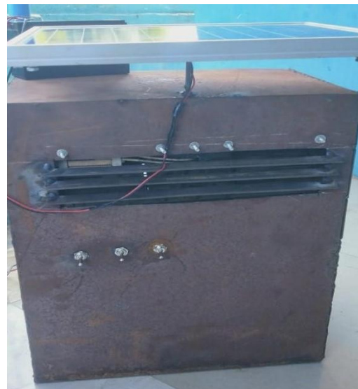
Fig:2 Solar Air Cooler with Heater
