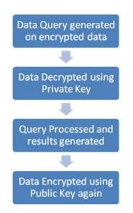
Figure I depicts how query on traditional encryption system allow Query Processing. The entire database needs to be encrypted to process any query. As discussed before, this takes significant amounts of time due to the slower rate of secure cryptographic techniques
