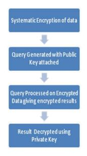
Figure II depicts the processed system of data encryption where the entire database is not encrypted as a whole but systematically encrypted to preserve some level of flexibility so as to allow query processing. This can be achieved by encrypting individual parts of data rather than the whole database
